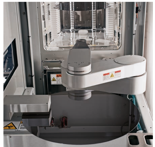
Automated precision: the handling robot feeds the XDV- \mu measuring system with wafers
