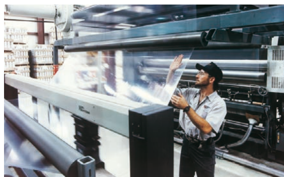
Measuring foil layer thicknesses in a running production line
